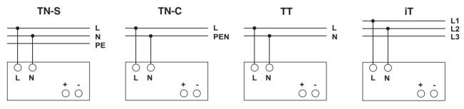
The 100 V AC ... 240 V AC connection is made using the L and N screw connections.
